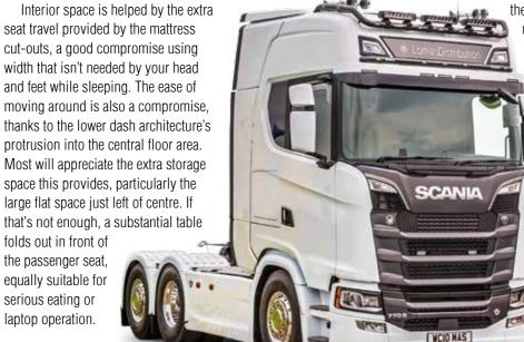
**VEHICLE SPECIFICATION** Manufacturer / Model Scania 770 S **Engine** Scania DC16 770 16.4-litre 759hp **Transmission** Scania Opticruise 12-speed Chassis 6x2 Cab type S High high-roof sleeper
